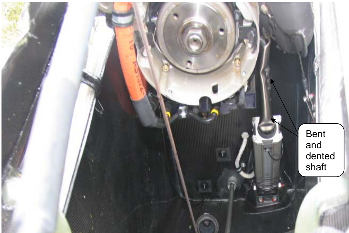
Photo 4: Bent extension/retraction shaft
