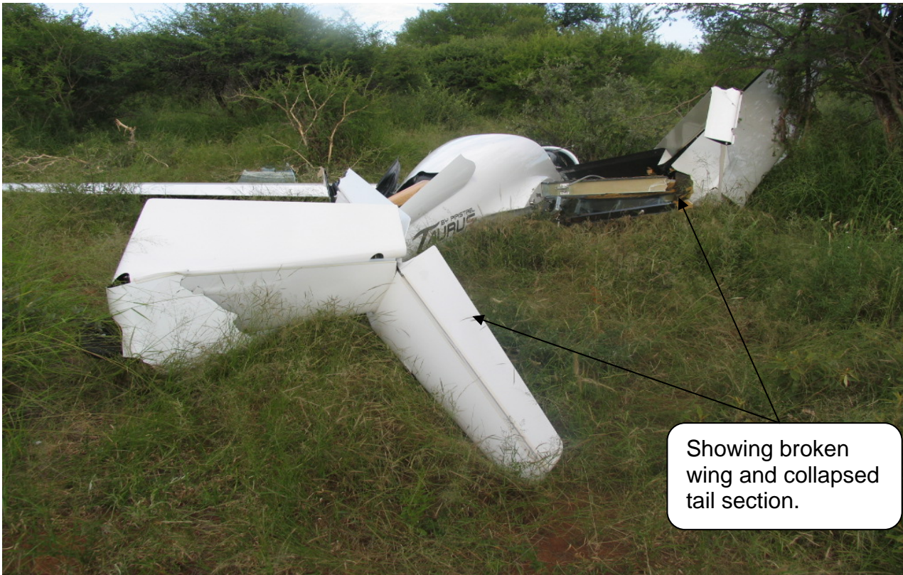
Photo 3: View from behind and aircraft damage
