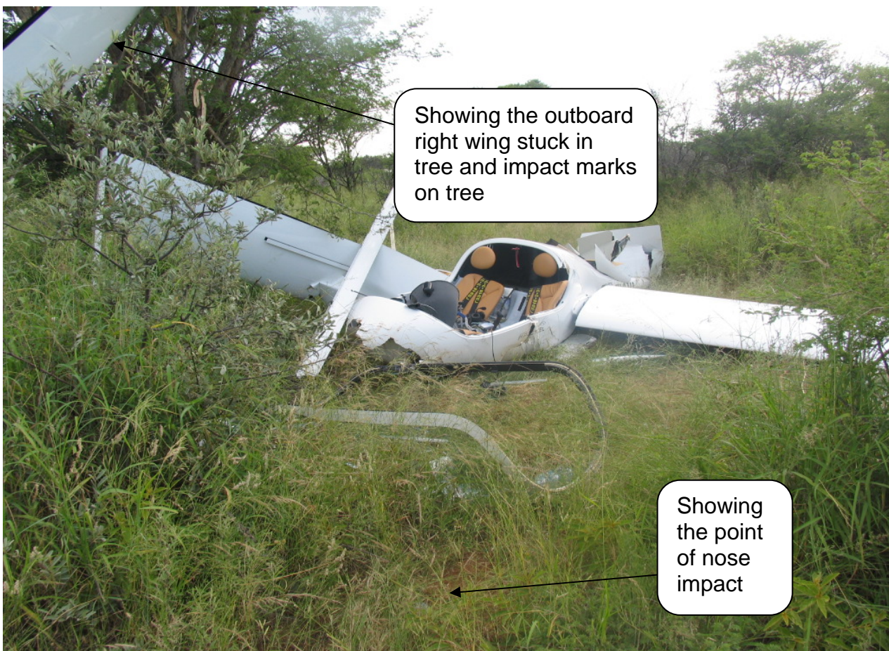
Photo 2: View from the front and impact marks
