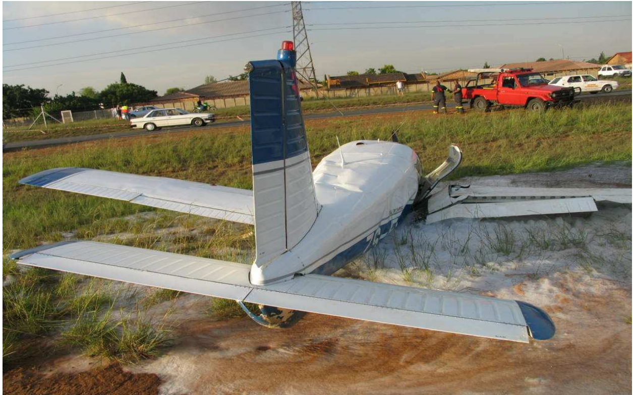
During the climb phase of the flight the aircraft collided with Eskom power lines and crash-landed
