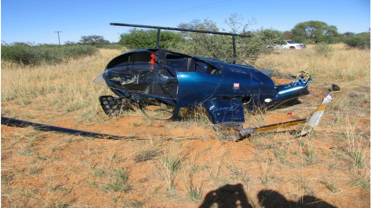
The aircraft collided with electrical wires.
