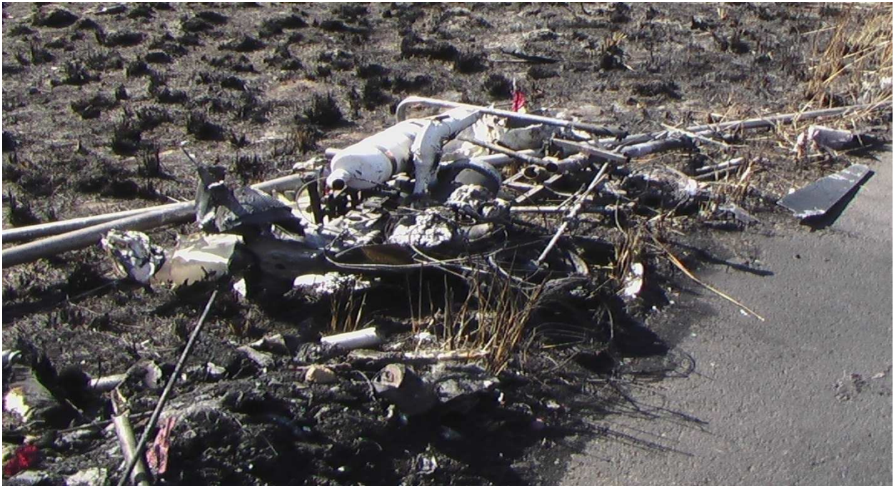
The aircraft collided with high tension wires spanned across a road.
