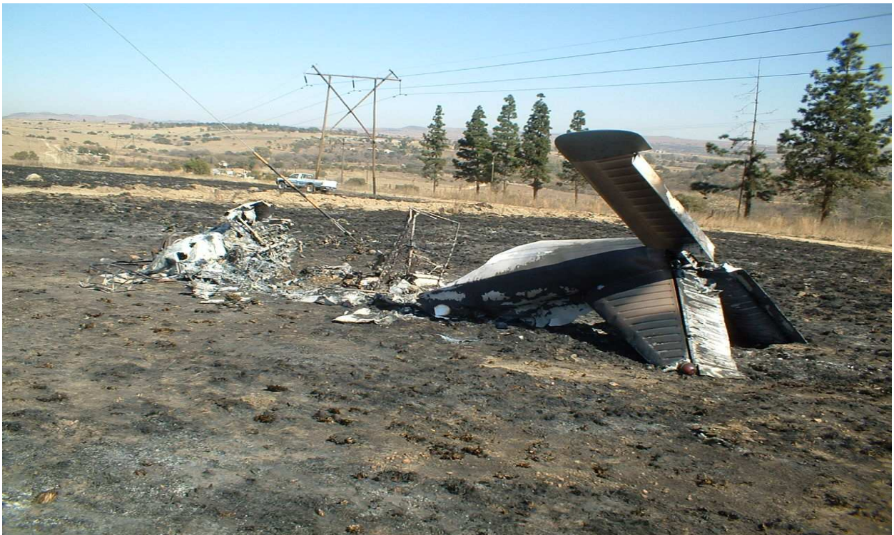
The pilot was low on the approach for landing and collided with high tension wires.
