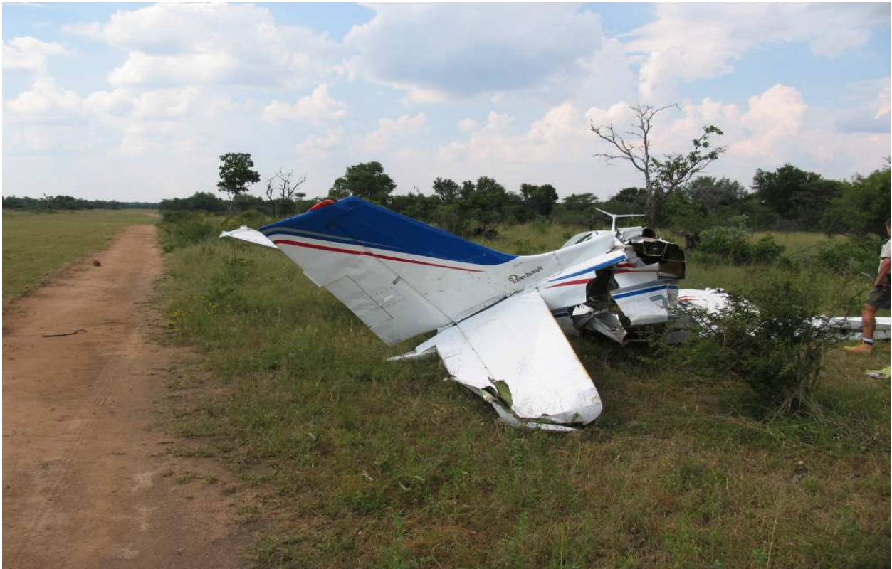
During the short final approach for landing at an unlicensed private runway, the aircraft collided with power lines and crashed on the right-hand side of the runway.
