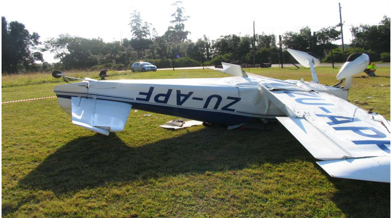
Aircraft collided with the power lines and telephone lines and crashed. Pilot failed to see power lines.
