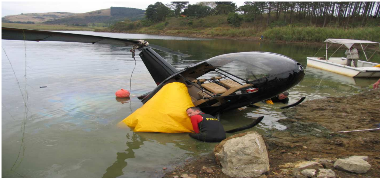
The helicopter collided with an electrical wire that was spanned across a dam.
