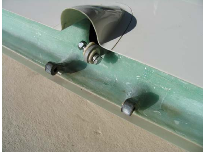
View of two of the hinges supporting the flapperon control surface.
