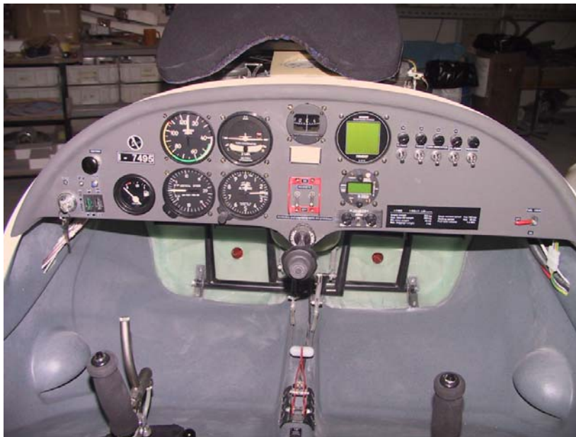
Conventional cockpit layout with the Vne indicated in red at 108 kts on the airspeed indicator.
