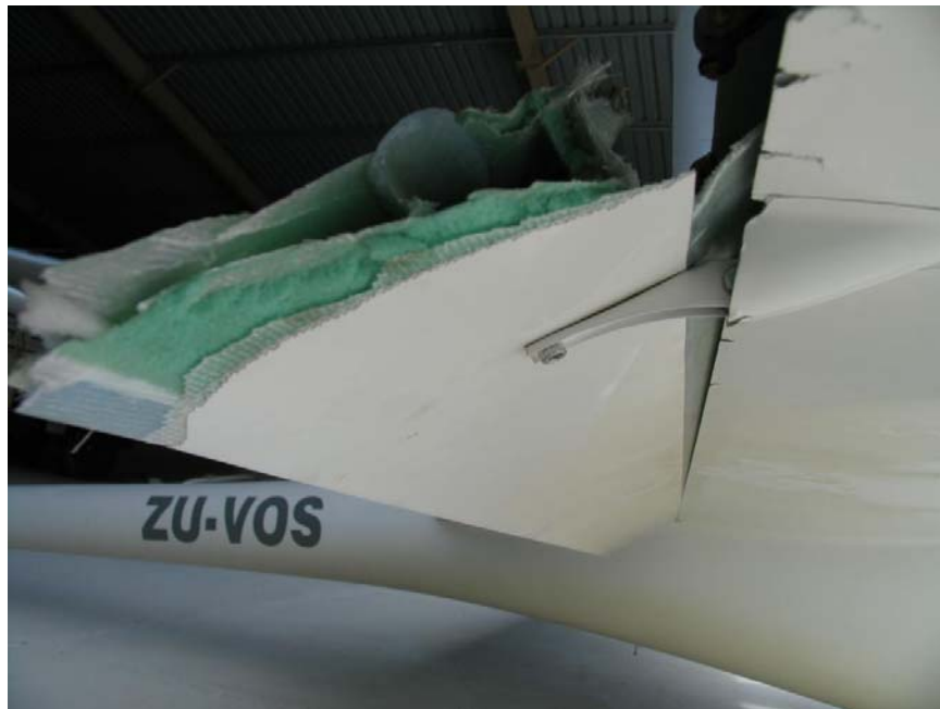
Section of flapperon, 1.58m in length, that remained attached to the wing structure.
