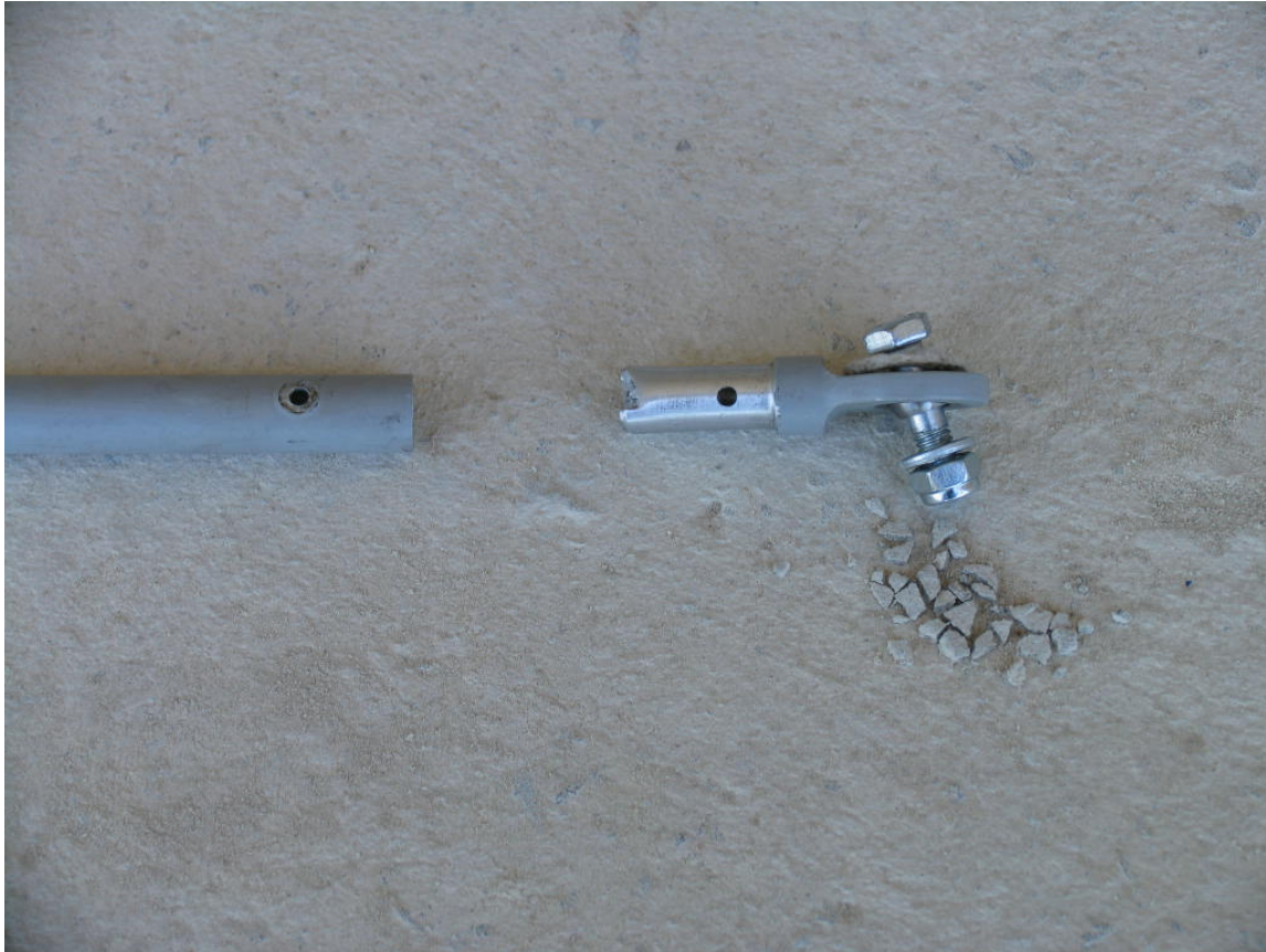
View of flapperon push/pull eyeball end, which was found detached.
