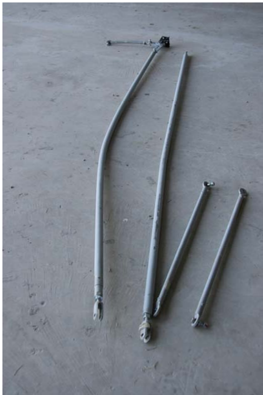
View of bent flapperon push-pull control rods.
