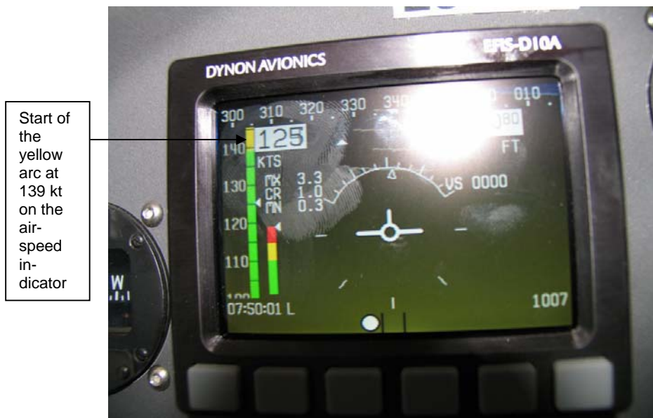
A view of the EFIS instrument displaying the airspeed indicator on the left-hand side.
