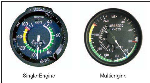
Figure 7-2. Airspeed limitations are depicted by colored arcs and radial lines.
