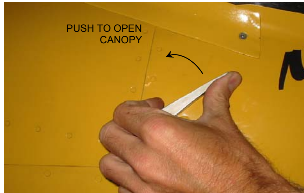
Figure 3 – Canopy Operation
