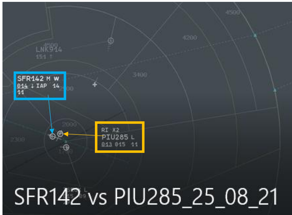
Figure 3: Safair142 and PIU285 at 07:25:08 hours, at which time the vertical separation was around 100ft and a lateral separation of around 0.2nm (370.4m).
