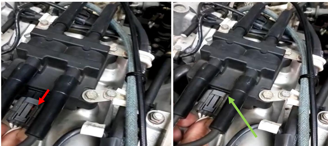
Figures 3/4: A disconnected ignition coil plug found on the engine post-accident (left) and the ignition coil plug fitted back onto the connector (right).
