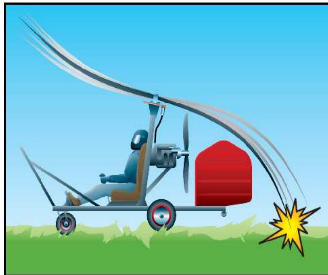
Figure 5: Taxiing too fast or gusting winds can cause blade flap in a slow-turning rotor. If not controlled, a rotor blade may strike the ground.
