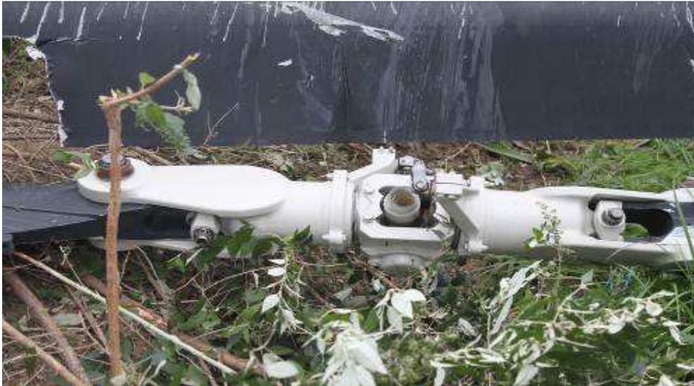
Figure 4: The main rotor that was sheared off the mast
