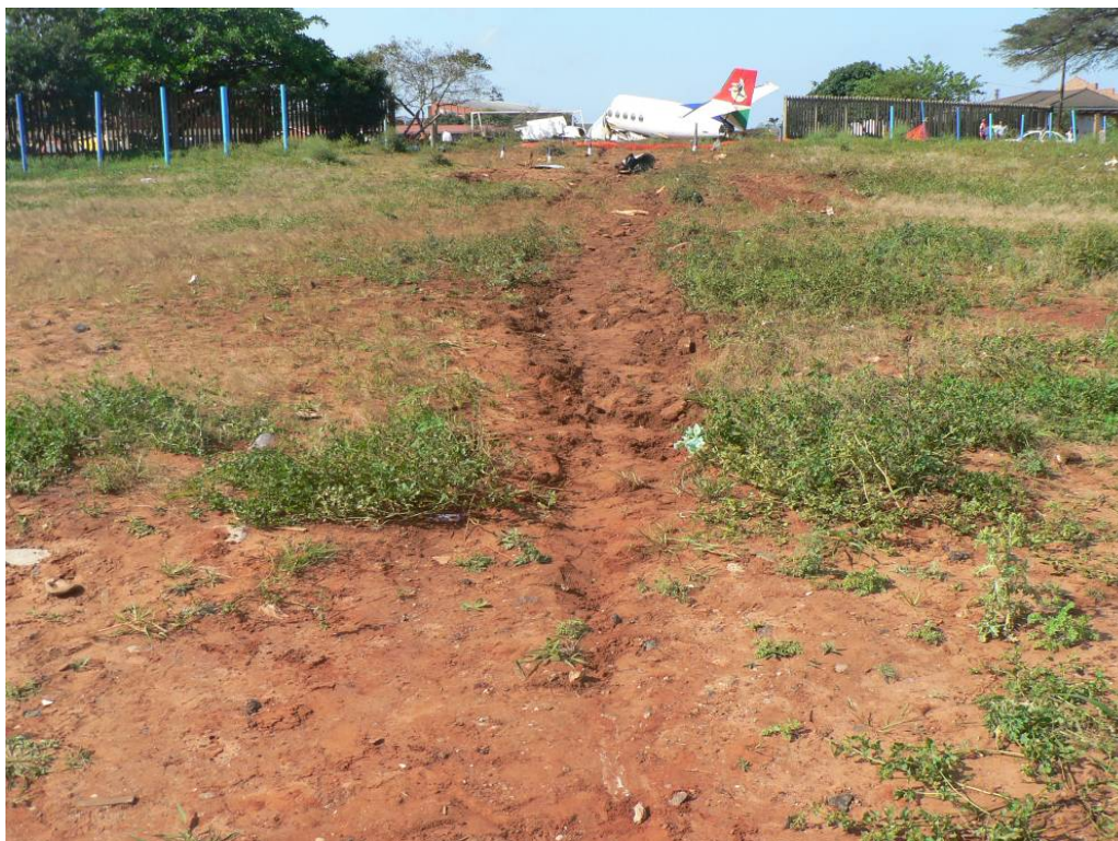
Figure 5. The first impact mark of the tail cone.
