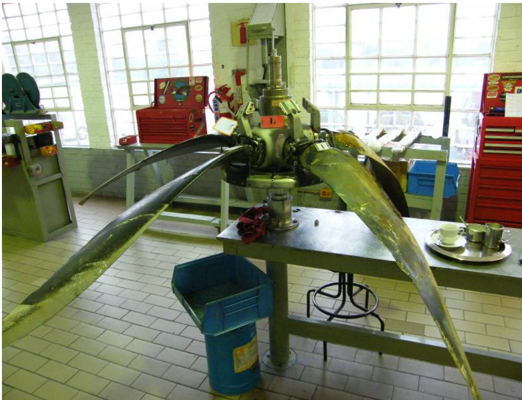
Figure 9. Damage to No. 1 propeller.
