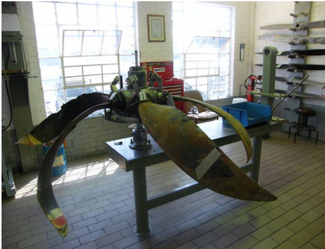
Figure 10. Damage to No. 2 propeller.
